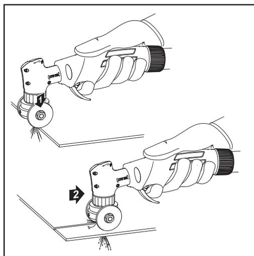
Fig. 5 Cutting with guide set, which is available as an optional extra
